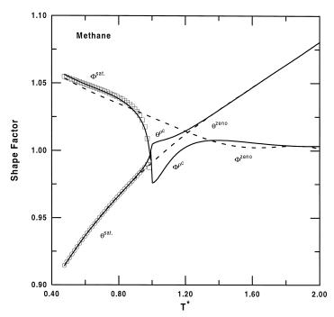
Fig. 2. Illustration of the lack of correspondence along the critical isochore and zeno line for methane. The dashed curves are the shape factors on the zeno line while the solid lines show values along the critical isochore.
