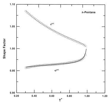
Fig. 1. Comparison of correlated subcritical n-pentane shape factors obtained with Eqs. (12) and (13) to exact values calculated with Eqs. (1) and (2).
