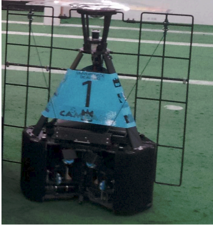
Figure 3: The goalie of the robotic soccer team CAMBADA with the Kinect sensor installed on its frontal part.
