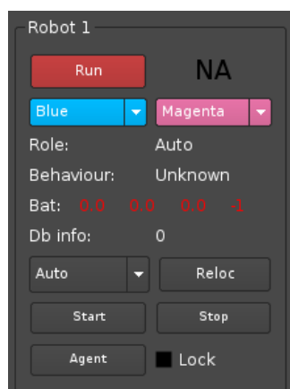
Fig. 2 - The RobotWidget module showing the information and the commands available for one robot.
