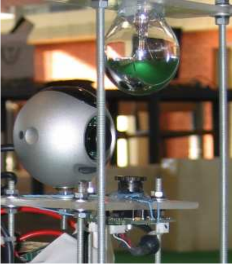
Fig. 4. The robot vision system in detail. Here we can see the configuration of the cameras. Note the position of the lamp, acting as a mirror for the OmniVision.
