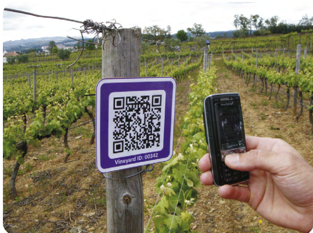
Fig. 1. Ubiquity in vineyard management practices. In this example, a cell phone and a bidimensional tag are used by a viticulturalist as an identification element to access, in situ , contextualized on-demand services, supplied, for example, by a knowledge-based data repository. Disease and pest checks, treatments, green harvesting, and other practices can be recorded in-field much more easier.
