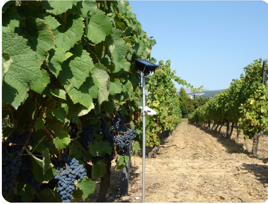
Fig. 11 – Photograph of an MPWiNodeZ device used in environment monitoring in a vineyard (air and soil temperature, solar radiation and relative humidity in this case).
