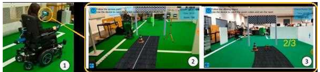
Figure 1. User experiencing the augmented reality serious game (ARSG): 1—set up used for controlling the robotic wheelchair; 2—following the white line in the middle of the road; 3—following the path of the moving object (car) until it stops.
