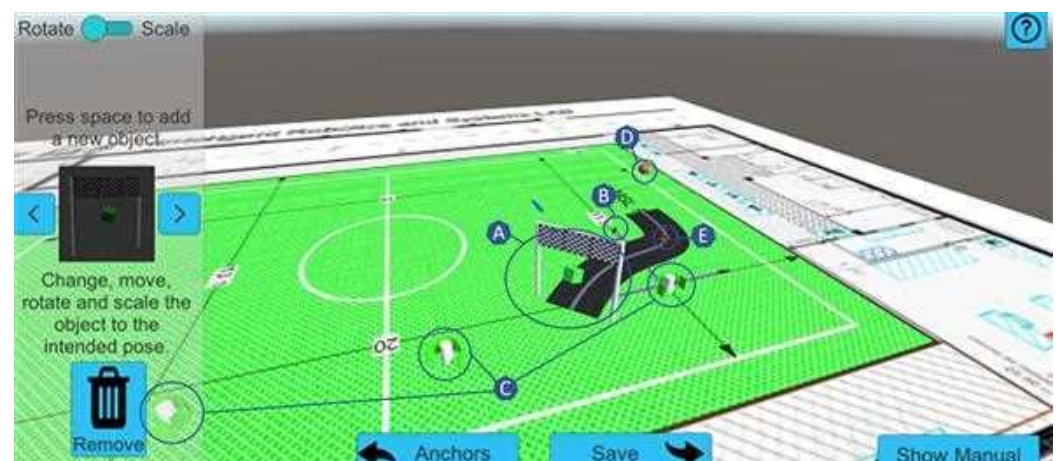
Figure 5. Configuration mode on a computer, illustrating how virtual objects can be positioned in a real-world environment. Overview: A—passage points; B—directional arrow; C—objects representing the cloud anchor locations; D—object representing the starting position; E—moving car.
