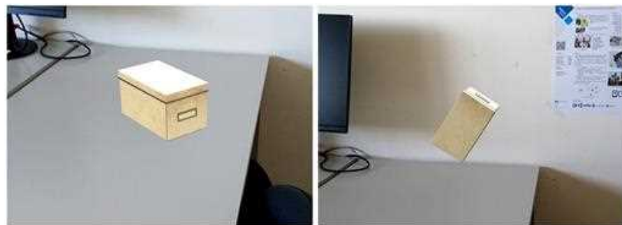
Figure 7. Placement of a virtual box onto a surface according to its normal vector. Depending on where the centre of the screen is aimed, the box base is placed parallel to the table ( left ) or to the wall ( right ) and in contact with the surfaces.
