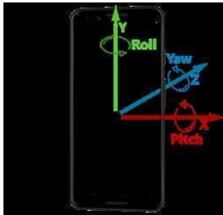
Figure 6. 3DOF of Rotation in a smartphone.
