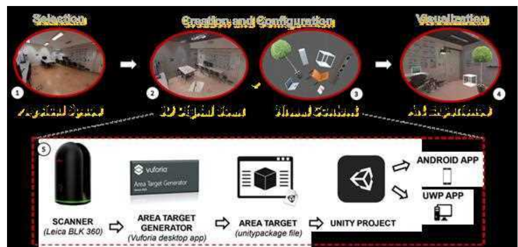
Figure 2. Creation process of pervasive AR experiences: 1. real-world environment; 2. reconstruction of the physical space; 3. integration of pre-existing augmented content according to the experience scope; 4. visualization of continuous AR-based content in the physical environment; 5. overview of the necessary steps to generate the experience.
