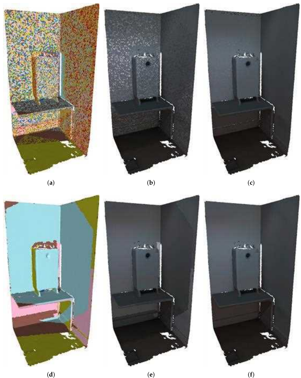
Figure 10. Textured meshes produced. (a) and (d) illustrate the result of the random selection and the selection based on the largest area of the projection, respectively. The color of each face is associated with the selected image, meaning that faces with the same color have the same selected image. The resultant textured mesh with random selection as the image selection technique is depicted in (b) using the original images, and in (c) using the color corrected images. The resultant textured mesh with image selection based on the largest area of the projection is depicted in (e) using the original images, and in (f) using the color corrected images
