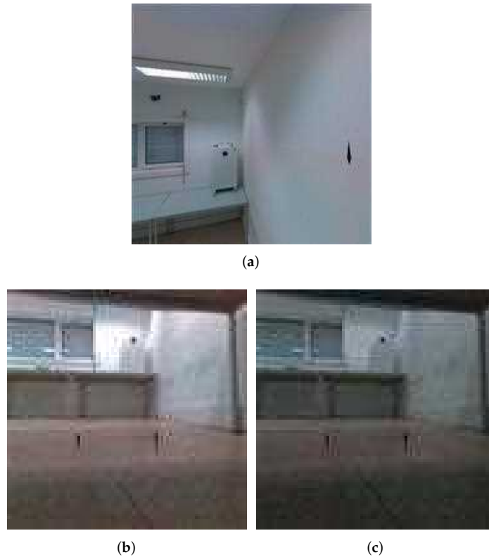
Figure 8. Example of the color correction for a pair of images: (a) Chosen reference camera (source image S ); (b) Original target image T ; (c) Color corrected target image \hat{T} .
