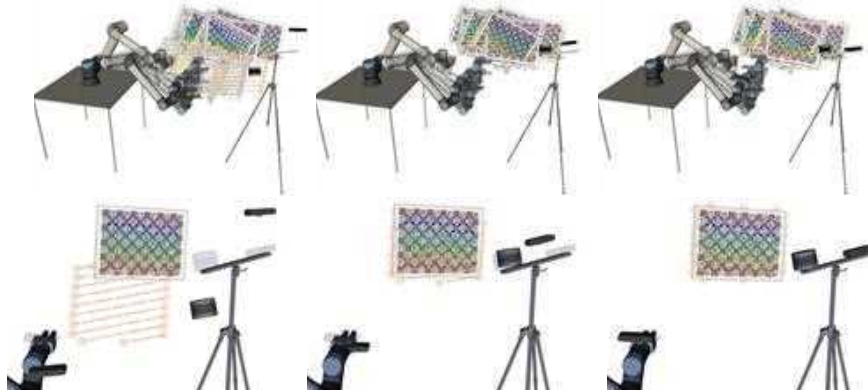
Figure 11: Visualizing the evolution of a calibration procedure from the initial estimate (left) to the solution (right). Top row shows all collections used in this calibration (different color for each collection). Bottom row shows a single collection and, in transparent mode, ground truth poses of the sensors (known because this dataset was generated in simulation).
