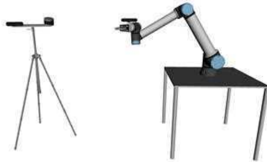
Figure 2: The Multi-Modal Test roBot (MMTBot), a simulated robotic system containing, from left to right in the figure: a RGB camera and a 3D LiDAR mounted on a tripod, and a second RGB camera assembled on the end effector of a robotic manipulator.
