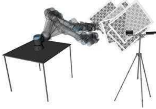
Figure 3: A dataset with multiple collections, each with a different configuration of the robotic arm and pose of the calibration pattern.
