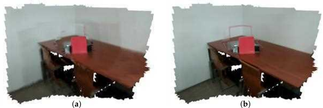
Figure 2. Using one or many images in texture mapping: (a) average-based approach; (b) winner-take-all approach. Images produced by OpenConstructor before final optimization (a) and after optimization (b).
