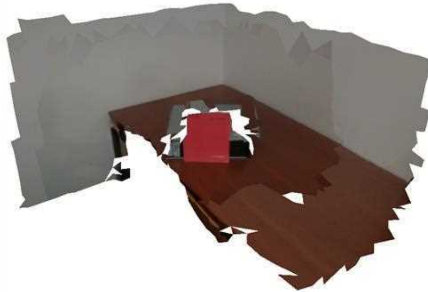
Figure 7. Textured mesh generated using the depth consistency algorithm. Notice that, in comparison with the standard winner-takes-all strategy displayed in Figure 2b, the red color (from the book) is not mapped on the wall.
