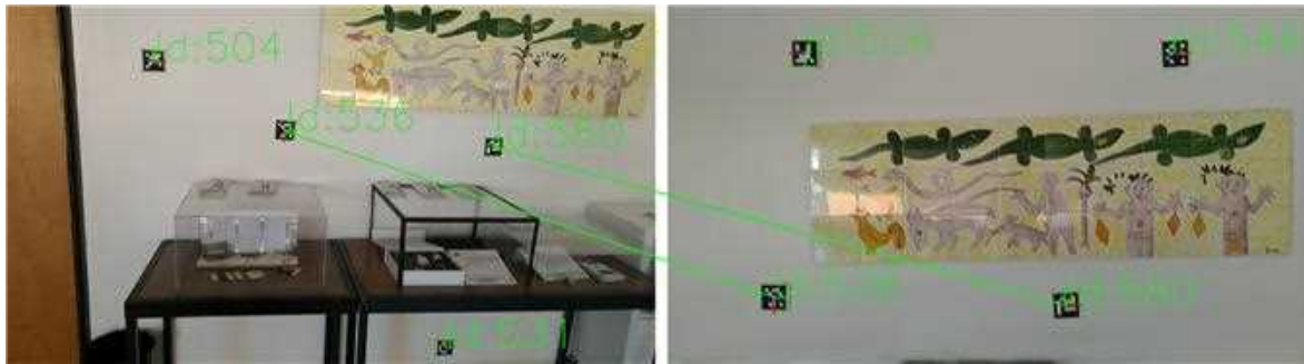
Figure 2. Detection and matching of aruco markers in a pair of captures.
