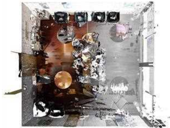
Figure 17. FARO laser scanned point cloud after downsampling.
