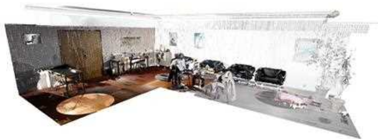
Figure 18. FARO laser scanned point cloud after downsampling and clipping.
