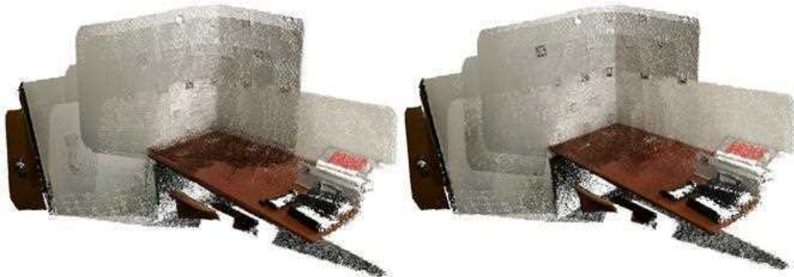
Figure 16. Point cloud coloured with texture obtained from restored images, no cross-inpainting: (left) before optimization; (right) after optimization.
