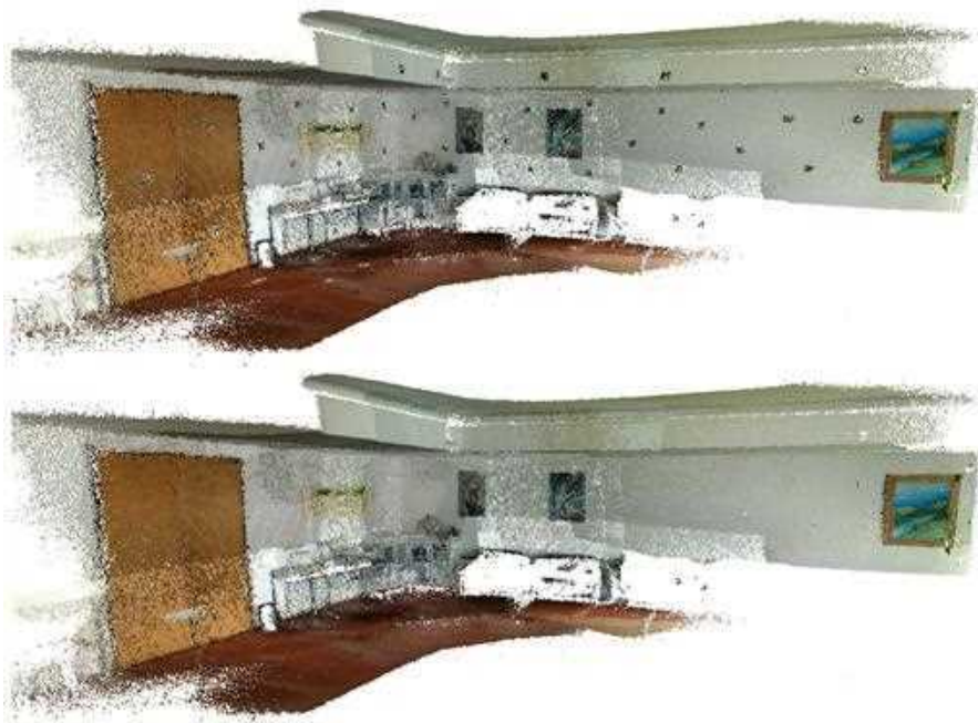
Figure 24. MeetingRoom dataset coloured with texture: (top) obtained from original images; (bottom) obtained from restored images.
