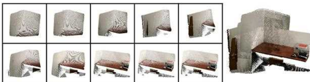
Figure 1. Example of registration of several point 3D point clouds to create a complete 3D model.
