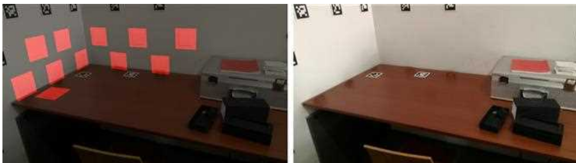
Figure 10. Example dataset image restoration improvement: (left) mask for the pixels to be replaced (based on enlarged 3D masks); (right) results with second blurring.
