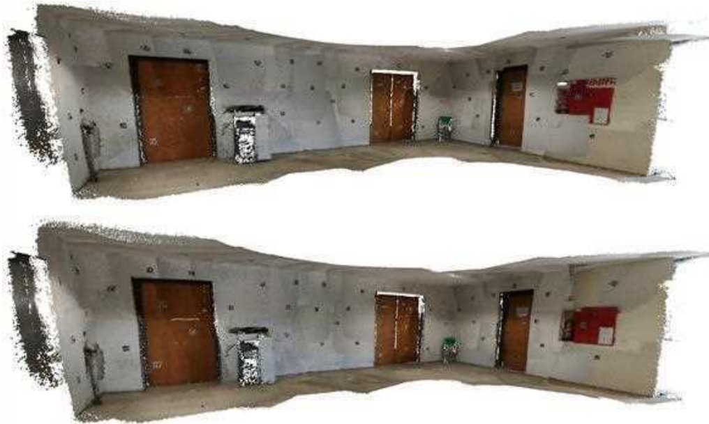
Figure 25. Lobby dataset coloured with texture obtained from original images: (top) Google Tango; (bottom) Our approach.
