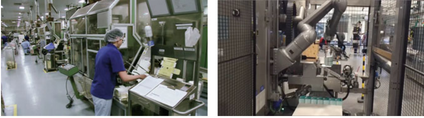
Fig. 7.1 State-of-the-art in the packaging industry. Blanks are feed manually (left image) or by a robotic arm in a cage (right image)
