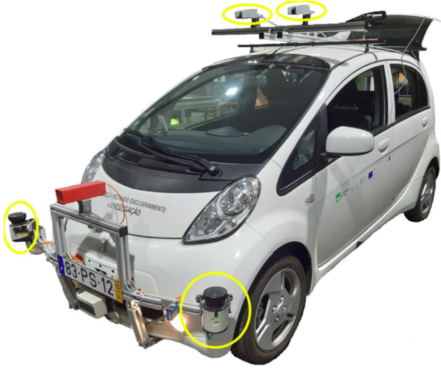
Fig. 7. ATLASCAR2: Autonomous vehicle from the Department of Mechanical Engineering of the University of Aveiro; the sensors are indicated by the Ellipses.
