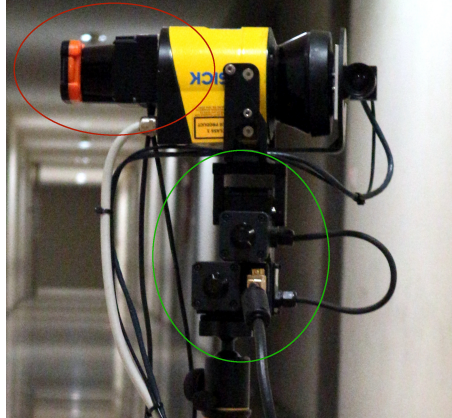
FIGURE 4: The lemonbot 3D scanner, used in this work. The LRF Hokuyo UTM30 is marked in red and the FLIR PTU-D46 is marked in green.
