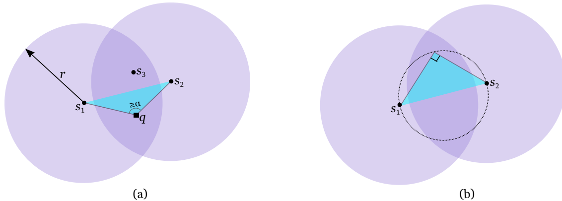
Figure 5.10: (a) Point q is \frac{\pi}{2} -covered because \angle(s_1, q, s_2) \geq \frac{\pi}{2} . (b) Blue wedge passing through s_1 and s_2 whose apex is located at the boundary of D_d(s_1, s_2) has a right angle.
