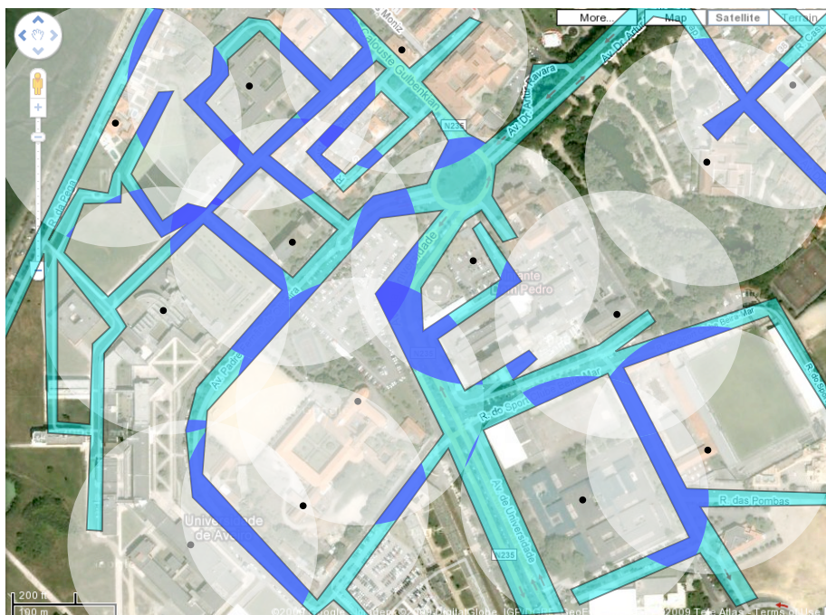
Figure 4.3: Regions covered by at least two antennas are shown in dark blue.
