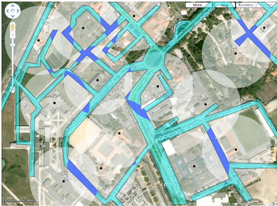
Figure 4.2: Regions within reach of at least two antennas are shown in dark blue.
