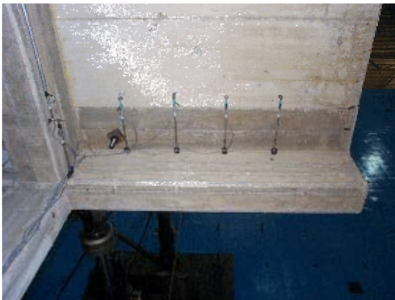
Figure A.22 - Instrumentation: slab (below)
