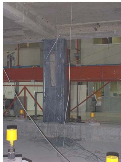
Figure A.33 - Instrumentation at the 1 st storey strong-column for the final capacity cyclic test
