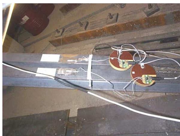
Figure A.50 - Bracing instrumentation (strain-gauges)
