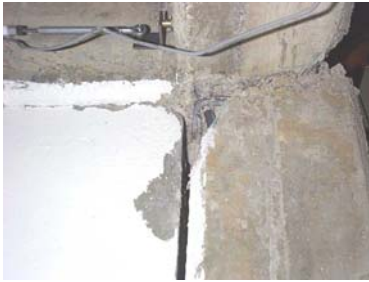
Figure B.25 - KB-cyclic test: damaged external columns ('shear-out')
