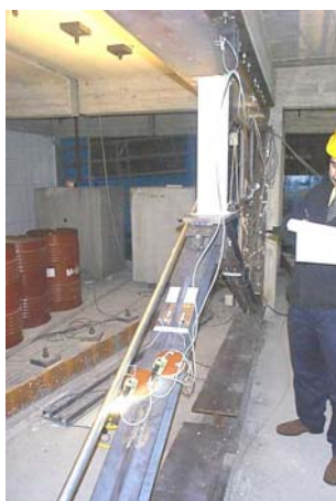
Figure A.50 - Bracing instrumentation (strain-gauges)
