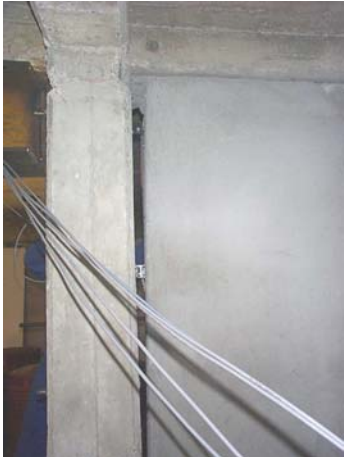
Figure B.25 - KB-cyclic test: damaged external columns ('shear-out')
