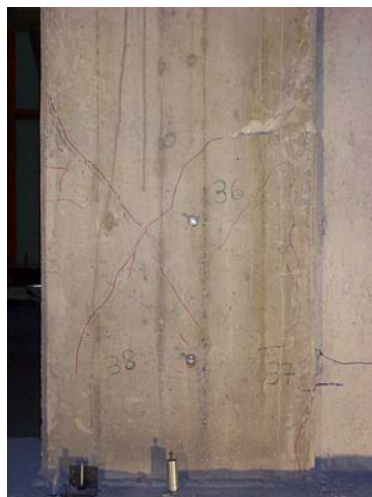
Figure A.55 - Damages on the first storey strong-column: frame A
