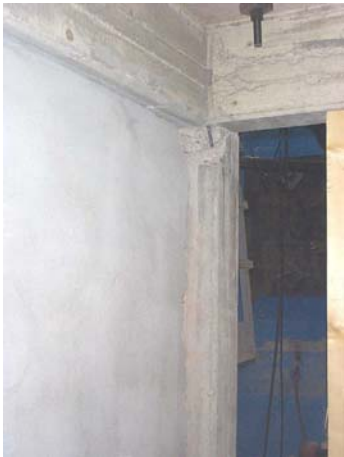
Figure B.25 - KB-cyclic test: damaged external columns ('shear-out')
