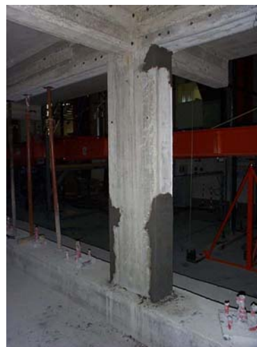
Figure A.55 - Damages on the first storey strong-column: frame A
