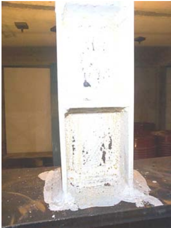
Figure B.24 - KB-cyclic test: damage pattern in the shear-link
