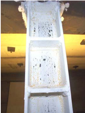
Figure B.24 - KB-cyclic test: damage pattern in the shear-link
