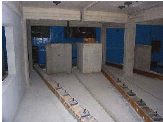
Figure A.17 - Additional loads (2.7 ton concrete blocks and 1.2 ton steel plates) and floor attachment steel bars system with pre-stressed connectors
