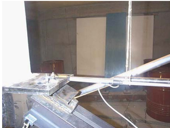
Figure A.51 - Instrumentation: relative displacement transducer (detail of the zone nearest to the shear-link)
