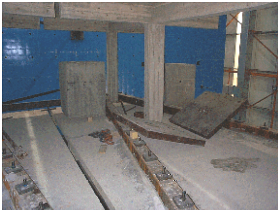
Figure A.17 - Additional loads (2.7 ton concrete blocks and 1.2 ton steel plates) and floor attachment steel bars system with pre-stressed connectors
