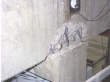
Figure B.26 - KB-cyclic test: details of the damaged external columns ('shear-out')
