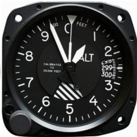
The original type of aircraft altimeter, with usability issues
